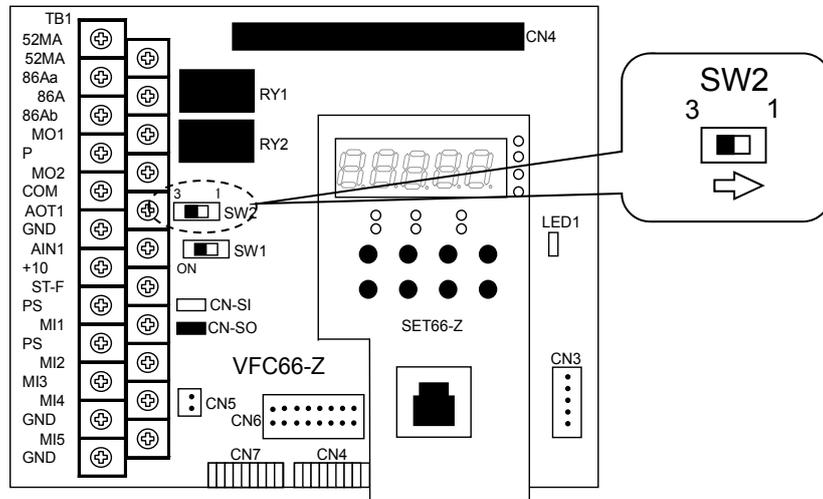
**1. When the analog output (1) characteristics selection is 6F speed (b-21 = -2)**
