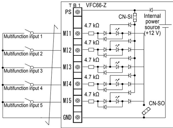
3. Sync mode (using the internal power source)
