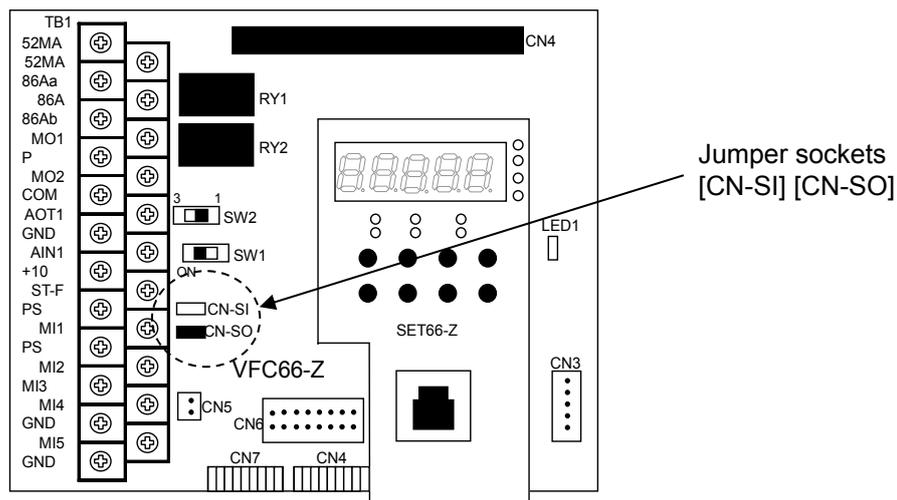
• When the jumper socket is [VFC66-Z CN-SI] and the internal power source is used
