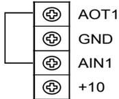
With VF66B (DC motor drive) turned off, open the front cover, and cause short circuit between (AOT1) and (AIN1) terminals of the terminal block [TB1] on the control print board [VFC66-Z] using the Phillips screwdriver (M3).
