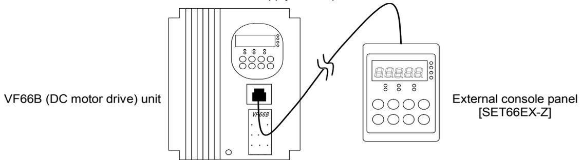
Connect the VF66B (DC motor drive) unit to the optional external console panel [SET66EX-Z].
