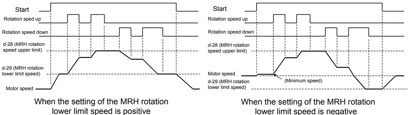
\* When a signal of the multifunction input preset speed selection or the speed commanding terminal block selection is input during MRH mode selection, the speed command of the multifunction input preset speed or the speed commanding terminal block takes priority, respectively.
