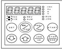
When the FNC (LED) on the console panel [SET66-Z] is turned off, press the [MONI/FNC] key to turn on the FNC (LED).
