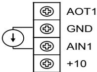
Turn off VF66B (DC motor drive), open the front cover, and connect the current power supply between (AIN1) and (GND) terminals of the terminal block [TB1] on the control print board [VFC66-Z] using the Phillips screwdriver (M3).
