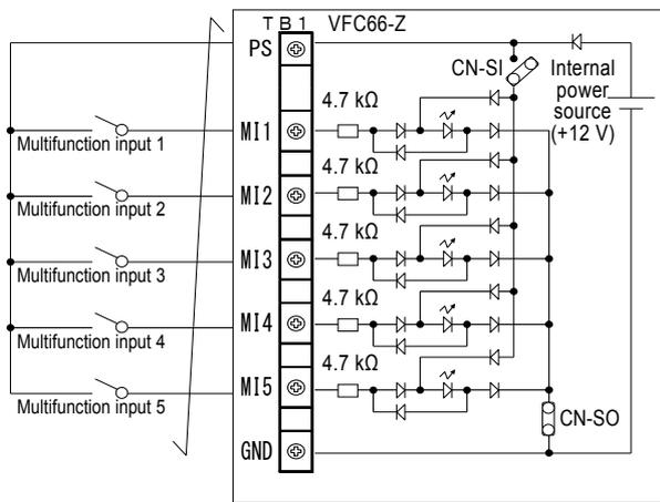
1. Source mode (using the internal power source)
