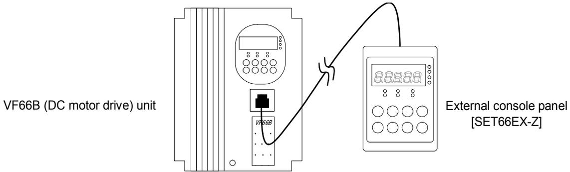
Connect the VF66B (DC motor drive) unit to the optional external console panel [SET66EX-Z].
