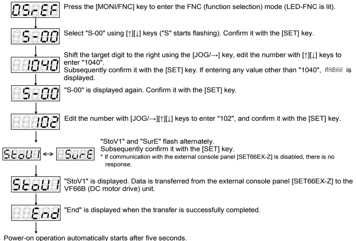
\* If normal communication fails during the data transfer, it is aborted with mode displayed, or **88888** flashes for 10 seconds and then the transfer is aborted. ⇒ To resume the transfer, follow the same procedure from the beginning again after mode is displayed.
