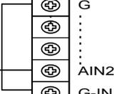
Turn off VF66B (DC motor drive), open the front cover, and cause short circuit between the (AIN2) terminal on the optional board and the (+10) terminal of terminal block [TB1] on the control print board [VFC66-Z] using the Phillips screwdriver (M3). Leave (G) and (G-IN) terminals on the optional board short circuited.
