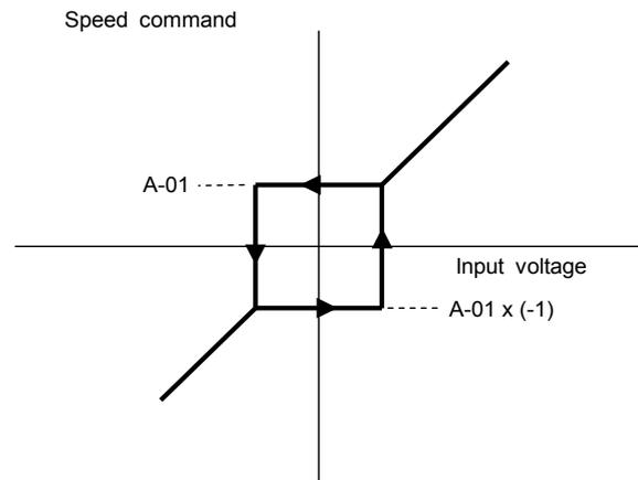
Figure 1-2 Hysteresis characteristics of minimum speed (A-01) around 0 V
