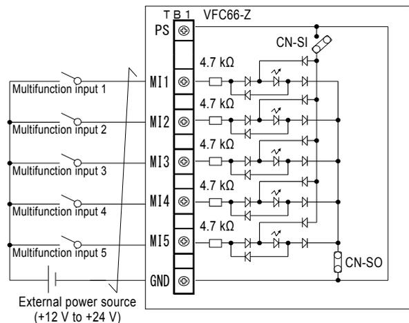
2. Source mode (using an external power source)
