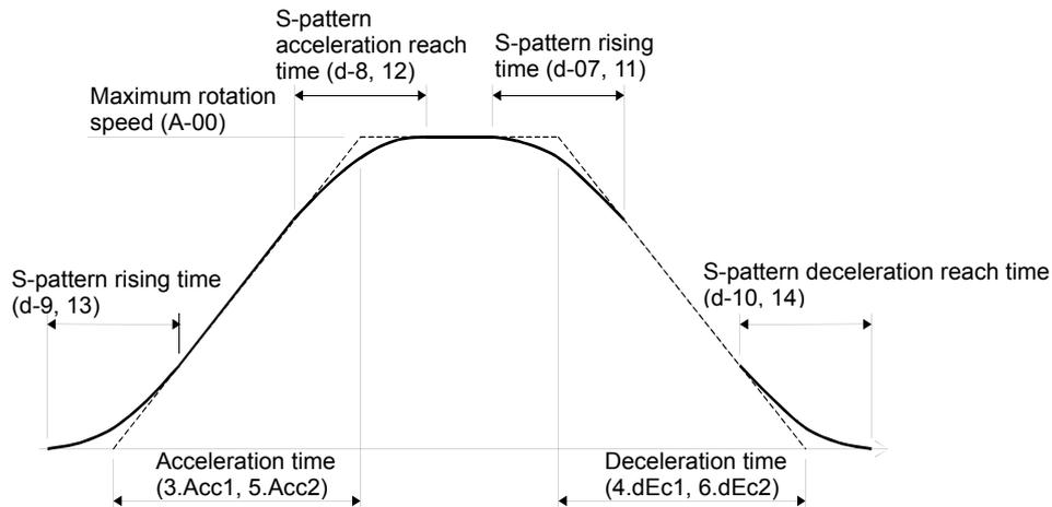
Time chart of acceleration/deceleration (s-pattern acceleration/deceleration)
