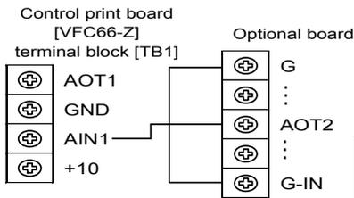
Turn off VF66B (DC motor drive), open the front cover, and cause short circuit between the (AOT2) terminal on the optional board and the (AIN1) terminal of the terminal block [TB1] on the control print board [VFC66-Z] using the Phillips screwdriver (M3). Cause short circuit between (G) and (G-OT) terminals on the optional board [IO66-Z] using the Phillips screwdriver (M3).
