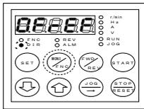
When the FNC (LED) on the console panel is turned on, press the [MONI/FNC] key to turn off the FNC (LED).
