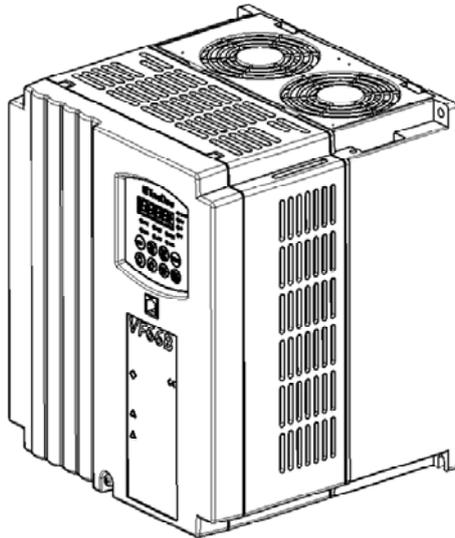
VF66B (DC motor drive) body
