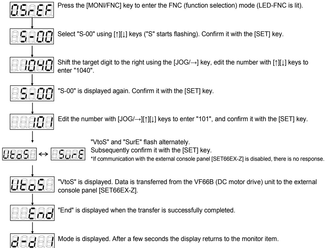
\* If normal communication fails during the data transfer, it is aborted with mode displayed, or flashes for 10 seconds and then the transfer is aborted.
