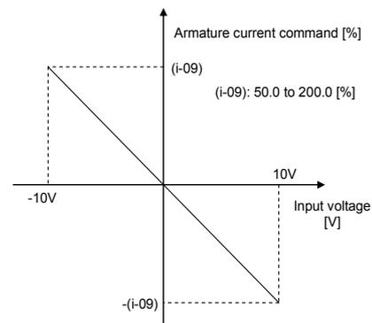
Analog input armature current command gain
