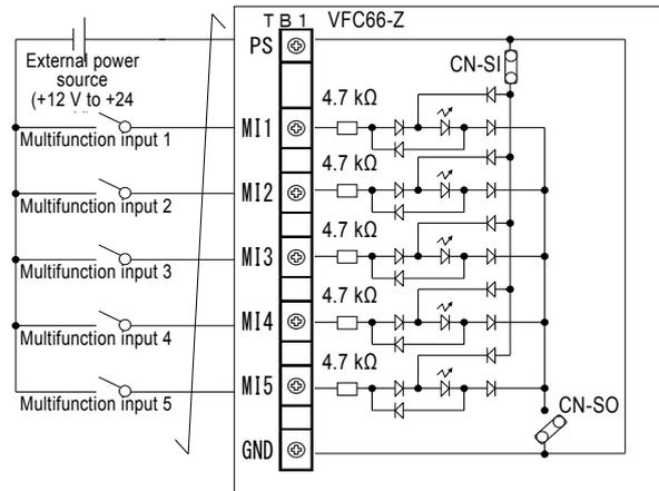
4. Sync mode (using an external power source)
